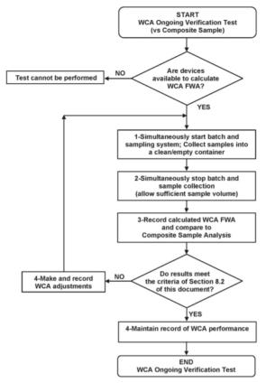
Figure 4—WCA FWA Reading Compared with Automatic Samples
