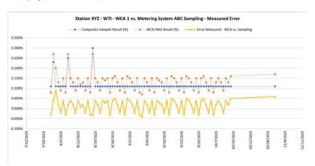
Figure C.1—Example WCA Ongoing Performance Verification Control Chart
