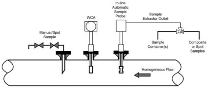
Figure A.2—Example In-line WCA Installation
